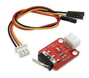
Simple circuit of Travel switch, collision module and integrated LED connecting to digital 13 interface to make collision flasher.
